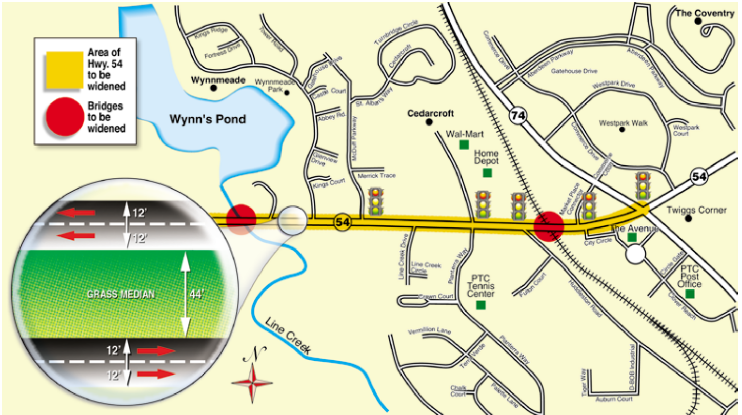
HWY. 54 ROAD WIDENING
